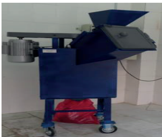
Figure 1. Chemical and mechanical device for designing and constructing a hospital waste disposal device
