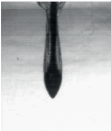
Figure 9. Body V-1, the speed of body entrance to the water is 4.5 m/s
