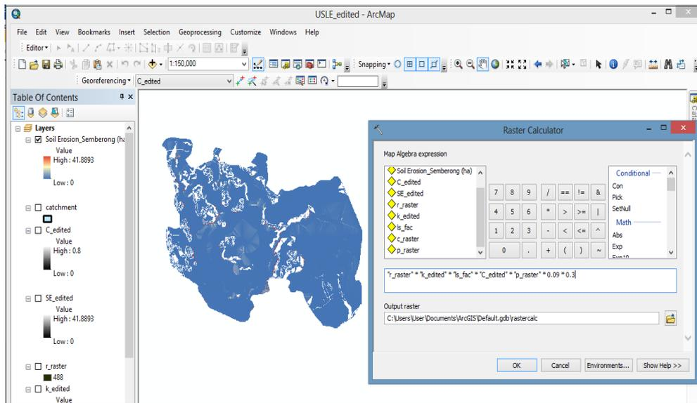
Figure 19. USLE calculation using raster calculator
