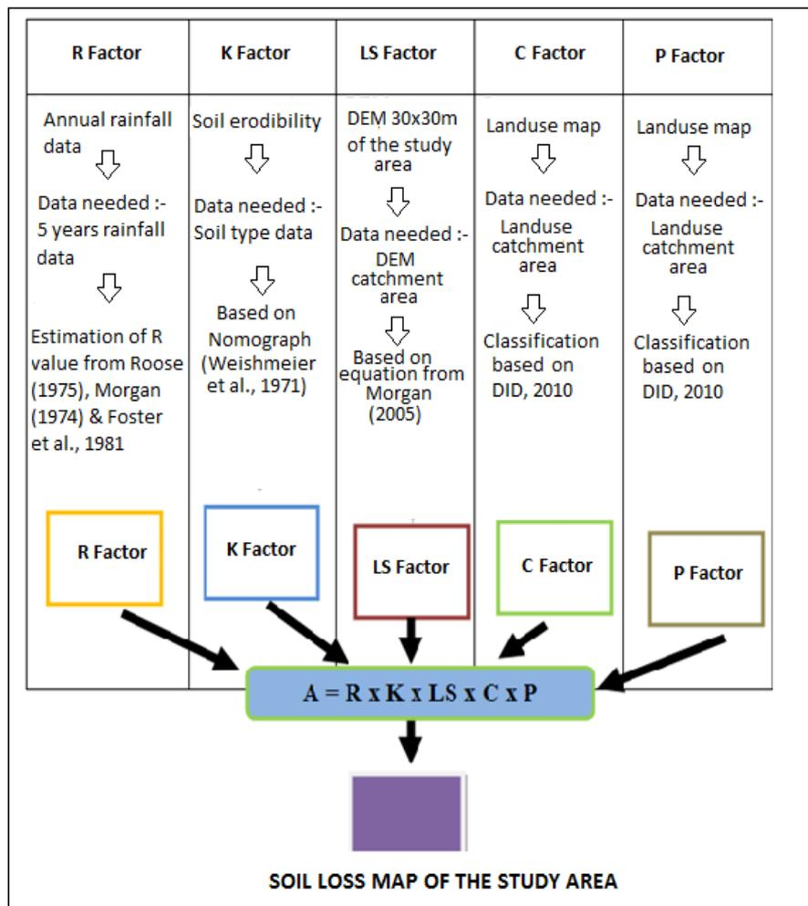
Figure 6. Workflow to determine all factors used in USLE (modified from Pillay and Rahaman, 2014). The result obtained will be multiplied by the sediment delivery ratio (SDR).
