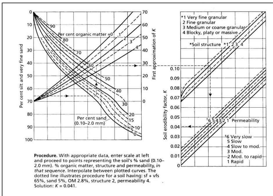
Figure 9. Nomographs to calculate soil erodibility (K) (t/ac.) x (100 ft.t. in/ac.hr) for Malaysia (Tew, 1999).
