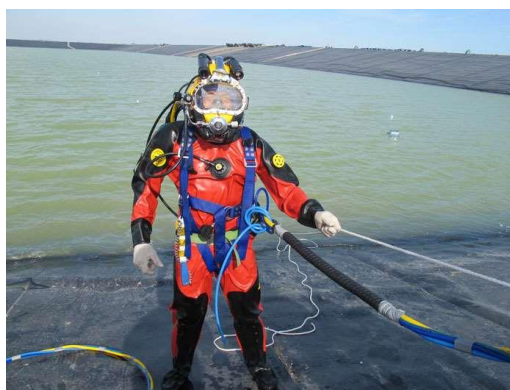
Figure 3. The recommended full diving suit for diving in polluted waters includes a full face cover, gloves attached to the suit, and also dry boots attached to the suit
