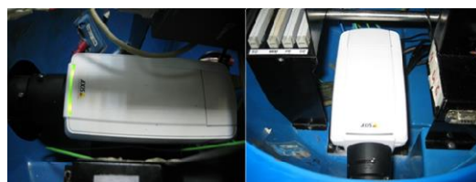
Figure 6. IP camera inside the head of the Aegir Submarine
