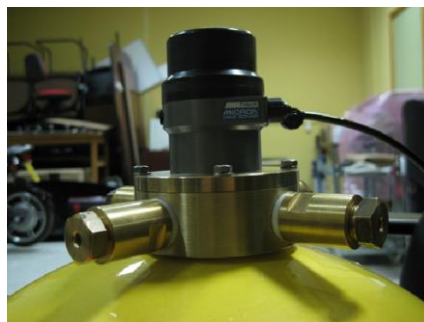
Figure 5. Image of the Micron DST sonar mounted on the head of the Aegir Submarine
